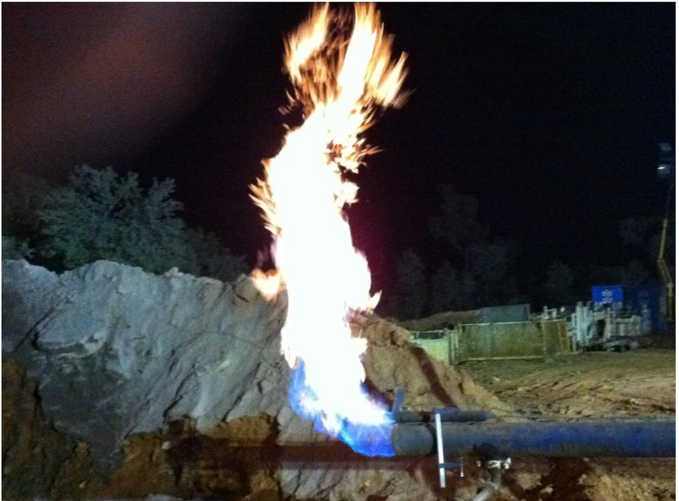
Picture of gas burning from the end of the 8" diameter blooie pipeline, venting Armour Energy's Cow Lagoon 1 well
