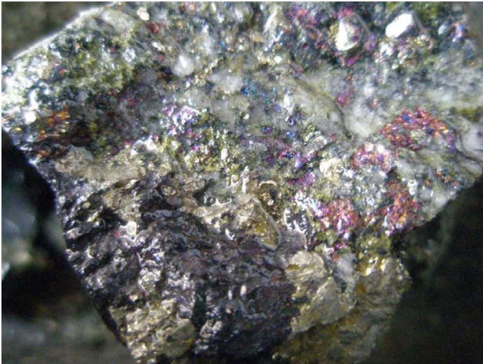
Figure 5: High grade Bornite-Chalcopyrite copper sulphides infilling veins Hole NS 3 (107 metres)
