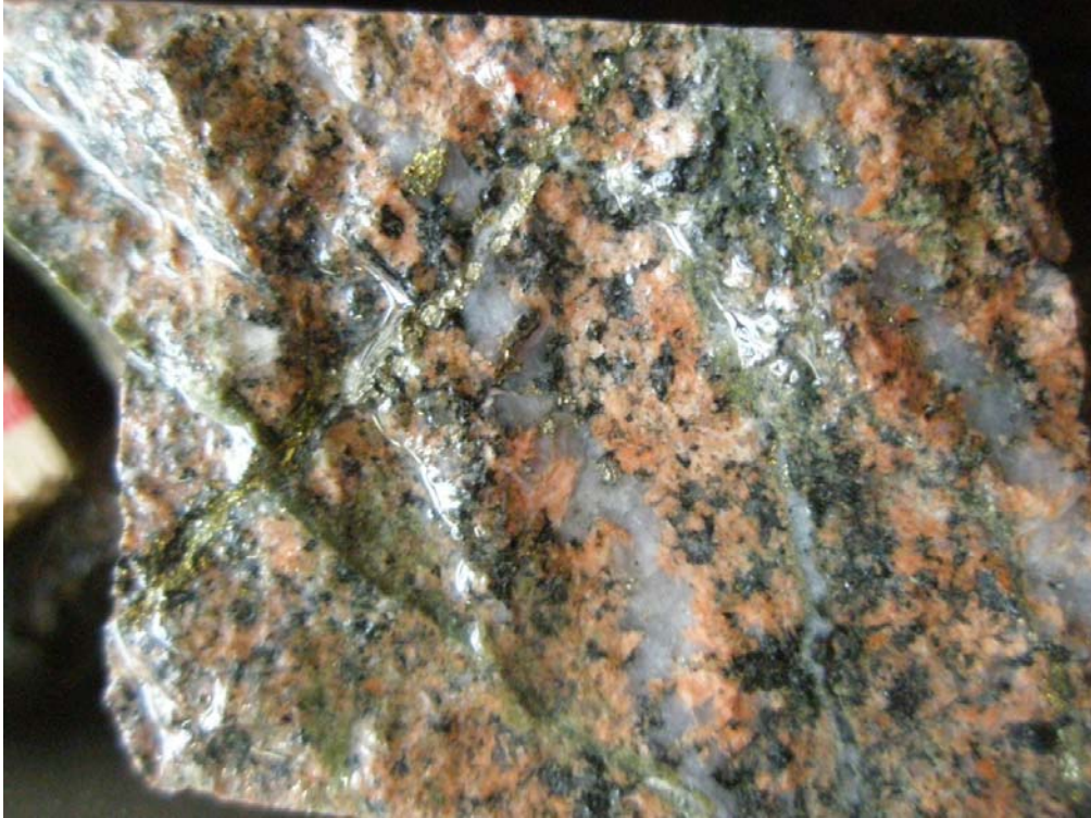
Figure 6: Low grade copper mineralization outside the high grade structures Hole NS 10 (62.2 metres)
