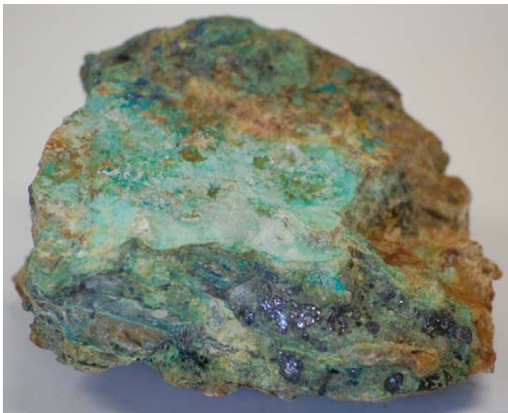
Figure 3: Silver-Copper-Lead rich rock chip sample from the Rossmore Silver Prospect workings. Major minerals include galena, malachite, azurite and siderite.
